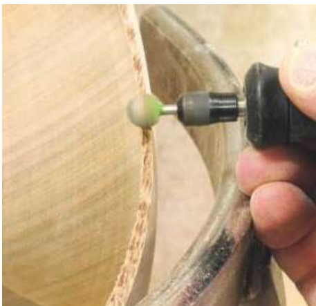
▲ Pic.25 Sorted. I made this fault a feature by adding a little texturing on the edge using a pineapple burr and a light burning with a small blow torch. This should create an interesting contrast with the natural wood, and nobody will know!
